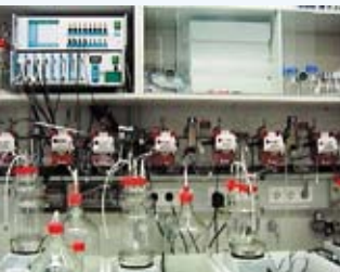
Fermenters for growing sulphur-oxidising bacteria
