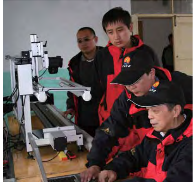
Figure 3. ICDP's optical core scanning system in use at the shore base.
